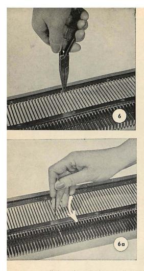
To remove the slide from the machine for cleaning, unscrew one of the two stop screws (15) at either end of the guide rails. Pull off the slide from the needle bed. This is a very simple operation. **Please do not use heavy household tools.**
