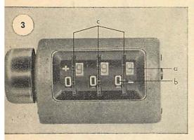
The row counter (20) shows how many rows you have knitted (fig. 3). The upper scale (a), marked with +, counts the rows. At the lower scale (b), marked with —, you can set the desired number of rows, then knit until the scale shows 000, when a bell will ring. The zero position, or the number of rows, can be set by turning upward the adjusting wheels on the right (c) of the check windows of the figures.
