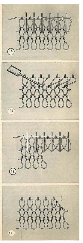
When the increasing is completed, the needles are brought into knitting position with the stitches lying behind the latches, and the yarn is placed around the sinker hook at the end of the row. Then, continue knitting.
