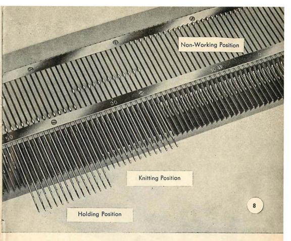
assume the correct working position. Whether you should use the needles in the center or at the sides of the machine, depends on the shape of your knitting. In general, you work in the middle of the machine, counting the needles evenly on either side of the center marked 0 on the upper rail. When knitting **without the wool feeder**, the ball of yarn which you have wound by hand or with the wool winder\*) is placed in a smooth container on the floor.
