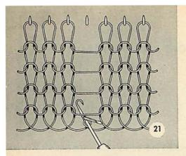
thread has been crocheted. Then, place the stitch on the latch needle again. Depending on whether the stitches are tight or loose, the rib holding device should be pulled down accordingly (either more, or less).
