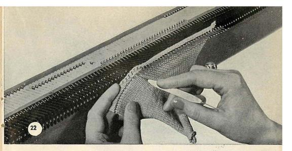
has been turned, the first row should be knitted slowly as the stitches are not yet under the sinker notches. It is advisable to pull the knitting down lightly, using your free hand\*).
