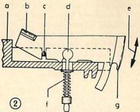
a) Needle bed, b) Sinker head, c) Sinker supporting shaft, d) Sinker pivot, e) Direction of travel, f) Sinker spring assembly, g) Sinker notch
