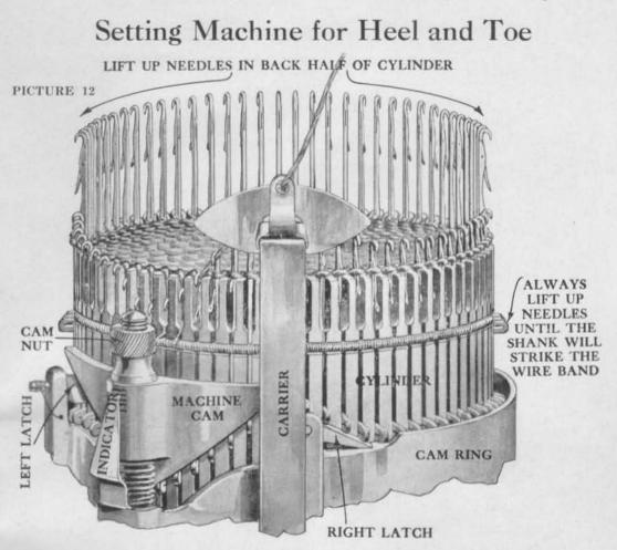
The Toe is made just the same as the Heel except in knitting the last two rounds of Toe at the finish. (Covered by instructions on Page 15.)
