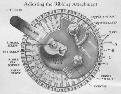
10. The machine is now set for ribbing. Turn the Crank forward about 20 times to see if everything is working right, and watch the need-les knitting.
