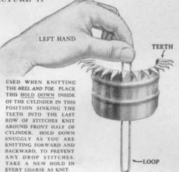
must be taken to hold down, with the thumb and fore-finger of the left hand resting down on top of the **teeth** on the ends of the **hold-down**. This action, if you press down hard enough, will prevent the first and last few needles, knit in each course backwards and forwards, from dropping stitches. After each course or two of knitting, lift up the **hold-down** and grasp a new set of stitches back of the needles and never allow the **teeth** to rest down on top of the **cylinder**.
