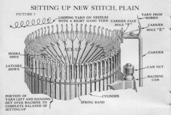
IMPORTANT Always have the Weights hanging on the knitting under the machine and lower Machine Cam sufficiently that the Weights will keep the stitches as formed from raising with the Needles or you will have trouble. When turning Crank always watch each Needle for first round of knitting clear around the Machine. When you are sure all needles are knitting, you can knit as fast as you like, but always be careful of knots in the yarn, going slowly while they knit in.
