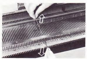
Note: If the Separators are in use, remove them before taking out the Needle Retainer.
