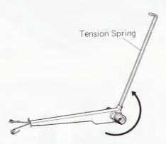
The Auto-Tension Rod can be installed on either side of the case handle. By using an additional Auto-Tension Complete (sold separately) you can knit four different coloured yarns without having the bothersome task of changing the yarns each time you wish to knit in a different colour.
