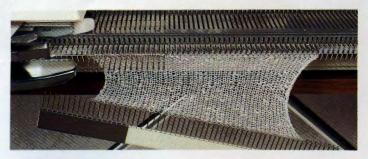
STEP No. 2. In order to avoid a hole forming between the needles that are knitting and the needles in HP, you must bring forward to HP one more needle and then knit one row.\* Repeat from \* to \* until all but the last group of needles are in HP.
