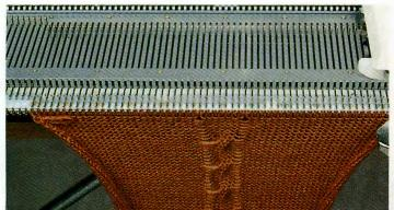
**STEP 2:** Remove the first group of cable stitches onto a Transfer Tool. Remove second group of Cable stitches onto a second Transfer Tool. Place the second group of Cable stitches onto the empty needles which previously held the first group, and vice versa.
