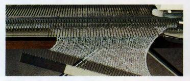
STEP No. 3. Set the Knitting Carriage to Normal (N) and knit one row. COL and all needles are in WP. The first wedge has been completed. Next, knit 9 rows, COR.\*\* Repeat from \*\* to \*\* to required length, cast off.
