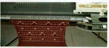
**STEP No. 1.** The main yarn is threaded as usual and the weaving yarn is best sat on the floor. Set for the first pattern row and take the knitting carriage across the needlebed. The needles are selected.
