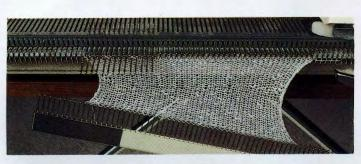
STEP No. 1. Cast on the required number of stitches and knit 10 rows ending with the Knitting Carriage at the right (COR)\*\* \*Push into Holding Position (HP) 4 needles at the left. Set the Knitting Carriage to "Hold" (H). Knit one row—Knitting Carriage is at the left (COL).
