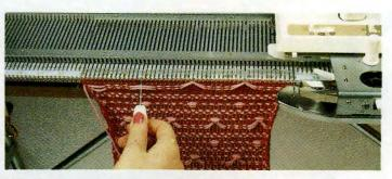
**STEP No. 4.** Long floats can be picked up and placed on the needles above, giving added interest to woven fabrics' ''pull-up''.
