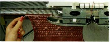
**STEP No. 2.** The weaving yarn is laid across the selected needles in the direction in which the carriage is going to travel. Hold the yarn lightly, letting the machine take the yarn it needs to form the stitch. The row is knitted, then the yarn is laid in the opposite direction.
