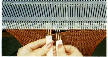
**STEP 3:** A good tip to help you and your machine is to bring the Cable needles forward to Holding Position (HP) after crossing — remember to set your machine to knit them back on the next row!
