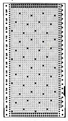
④ Finally, mark the arrows on the left side of the card to tell you when to use the Knitting Carriage.
