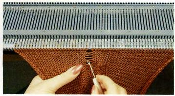
METHOD C—WORKING CABLES ON THE MAIN BED ASSISTED BY THE RIBBER
