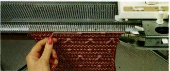
**STEP No. 3.** It is possible to create different textures and patterns by using the "Weaving Winding method", winding the yarn around groups of selected needles at regular intervals.
