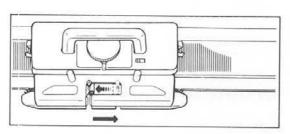
The Yarn Feeder moves during knitting. After aligning needles, check that the Yarn Feeder is at the left side. If it is not, move the Carriage a little more to the right.
