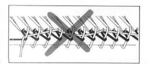
If the Ravel Cord is caught on the needle hook, the cast-on will not work correctly.
