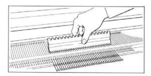
Using the Needle Pusher, align the needles in D position as shown.
