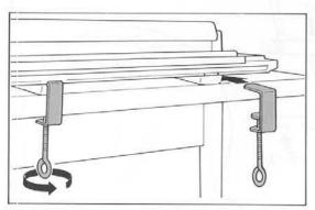
Place the machine on the table with its Carrying Handle away from you, and open the machine as illustrated above.
