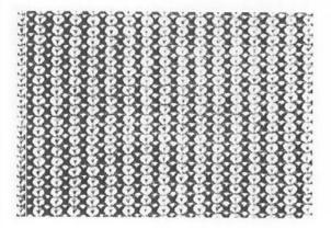
Tuck stitch patterns or slip stitch patterns can be knitted using yarns of different colours.
