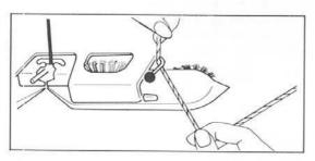
Place the weaving yarn inside the Holder on the leading side of the Carriage.
