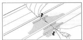
Push the damaged needles to D position. Close the latch and press the needle down. The shank will come out of the needle bed.
