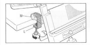
With Knitter Clamps "L", secure foot of Push-up Cams "M" on table.
