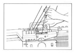
If more than three yarns are used, the Auto-Tension may not be able to take up slack on the yarn properly. In this case, slightly pull up the yarn above the Yarn Feeder, and also to correct possible entanglement of the yarns.
