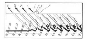
Push the needles by hand back to B position one by one, starting with the inner needle, and working to the outer edge.
