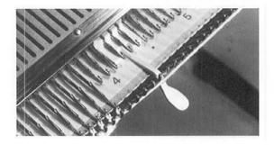
Open the latches of the 4th, 5th and 6th needles beyond the needles in B position.
