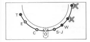
Check the setting of the Cam Lever. It should be set at "O" before mounting the Ribber Arm, never at F (FAIR ISLE) or L (PUNCH LACE).
