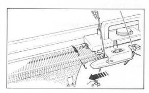
Holding the weaving yarn under the Arm, push the first knitting needle into D position, and then move the Carriage to the other side.
