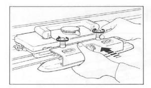
Loosen the two Arm Nuts, and insert the Arm under them.
