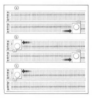
When stitches on full length float, push needles to C position using P Carriage (without P Presser) and knit.
