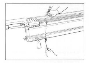
12. Hang the knot of the three yarns between both needle beds at the left side. Insert Hook Tool from underneath and catch the knot.
