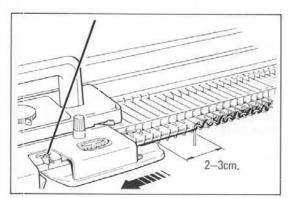
Ensure that the Arm has passed the last knitting needle by approximately  $2\mbox{--}3\mbox{cm}.$
