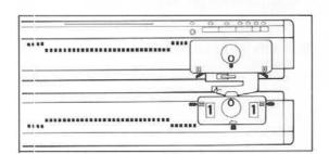
Arrange the needles for Double Rib and move the Carriage 2—3 times and leave it at the right side.
