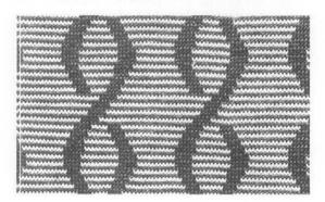
Double Jacquard — a fabric knitted with the use of the Pattern Card, and having no floats of yarn on its back.
