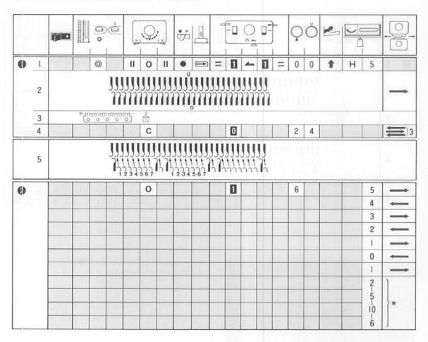
\* Knit swinging the Ribber by 1 pitch on every row to the extreme right, and then to the extreme left, to make zigzag pattern.
