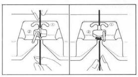
Guide the yarn into Yarn Feeder  $\odot$  , and holding the yarn end with your hand, close the Gate.
