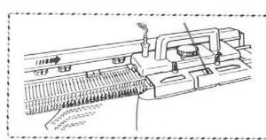
In lace knitting, all shaping must be done on the side opposite to the Carriage. The Point Cam must be moved to its new position (2 stitches in from the edge of the knitting) before knitting the next row.
