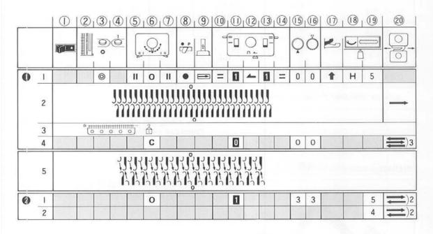
If the diagram shown is given beside the needle arrangement diagram in the Operation Table, set the Point Cams and Needle-1 Cam in the same step.
