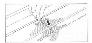
To replace a new needle (see NOTE), open its latch and slide it into the Needle Bed groove until the hook comes out of the front opening of the Needle Bed.
