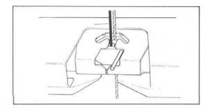
Two different colour yarns are knitted together. One yarn appears on one side whilst the second yarn appears on the other side of the fabric.
