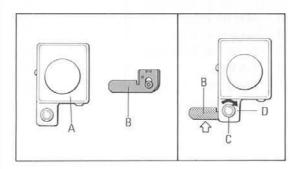
In drive lace knitting, use P Carriage "A" without P Presser "B". In pile knitting, use P Carriage "A" with P Presser "B" attached. Place P Presser "B" underneath Arm "C" and secure with fastening screw "D".
