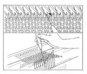
Ensure all stitches are in the needle hooks and the needles are in B position.
