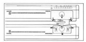
Move Carriage 2—3 times to align needles in B position finishing with Carriage at the right.
