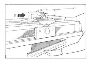
Holding Cast-on Comb, move Carriage once across needles.
