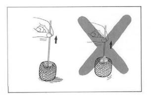
When yarn is rewound, ensure that the yarn end comes out freely without lifting the ball from the table.
