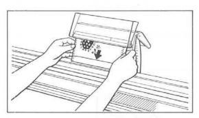
Insert the bottom end of the Pattern Card into the Card Slot.
