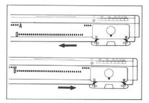
Slowly move the Carriage across the needles, and the needles will align in B position.
