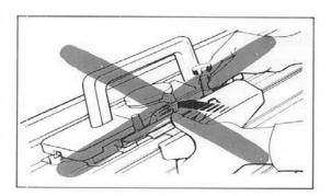
IF THE RIBBER HAS ALREADY BEEN CONNECTED WITH THE KNITTER, follow the instructions given below to use the Lace Carriage on the Knitter.
