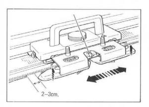
Set the Weaving Knobs back to O. Move the Carriage back and forth to knit stockinet.
