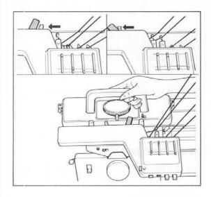
15. For main knitting set both Stitch Dials to 4 and move Carriage from the right to the left till Driving Lever hits Feeding Lever and yarn changing is completed. When yarn changing is accomplished, a click is heard.
