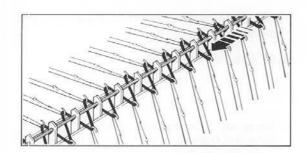
(3) Insert Wire through holes of Cast-on Comb teeth.
