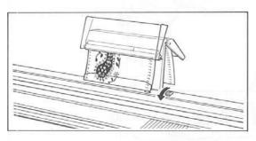
Using the Card Dial insert the Card further into the Slot and set it to the starting line.
