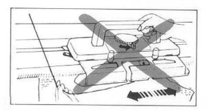
When the yarn is removed from the Yarn Feeder, DO NOT move the Carriage with the Cam Lever set at "L" or "O", as the fabric will be released from the needles.
