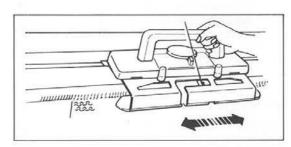
Cast-on (open edge) is completed. Continue to knit about 30 rows by moving the Carriage back and forth.
