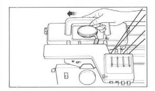
Start knitting from the right to the left till Driving Lever hits Feeding Lever to change the yarn every two rows.
