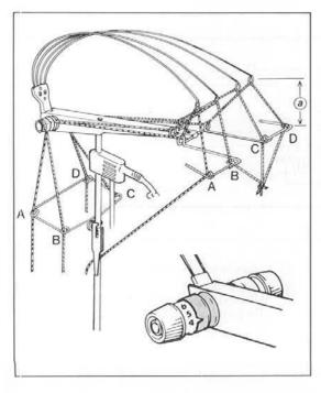
Thread four yarns of different colours into Auto-Tension. Important: follow the threading diagram exactly.
