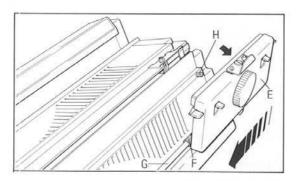
Take Ribber Carriage "E", and fit its pipe "F" on the Ribber Rail "G" from the right side.
