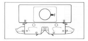
Thread the contrast yarn through the Auto-Tension and into Yarn Feeder  $\odot$  as shown opposite.
