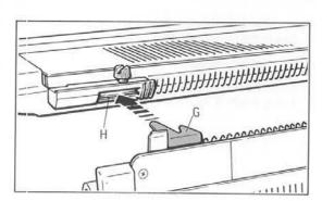
Hold Ribber with both hands and insert Ribber Joiners "G" on both sides into slots of Auxiliary Pieces "H".
