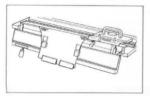
To knit the lace fabric with the Ribber attached, drop the Ribber to its lowest position and cover the needle bed.
