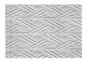
A selected needle remains inactive and the yarn passes in front of the needle. Non-selected needles knit stockinet.
