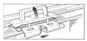
3. With the top of the Carriage up, move the Carriage in the direction it was going till it gets clear of the fabric.
