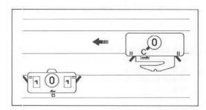
7. On Knitter Carriage, set Cam Lever to "C" (CIRCULAR). Remove yarn A from Yarn Clip and thread it into Yarn Feeder. Holding the yarn underneath the machine, move Knitter Carriage from the right to the left without knitting and connect it to the Ribber Carriage.
