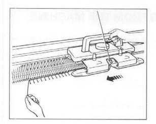
Hold the yarn at the left side of the needles, and make sure that the latches of the needles in D position are open.
