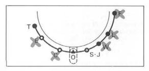
14. With the Cam Lever at the position you desire (0, T or S), start to knit changing yarns by pushing the Holder Buttons at the row you desire.
