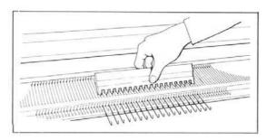
Using the Needle Pusher, push every 2nd needle from B to D position.
