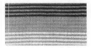
Using the Yarn Changer, but without using the Pattern Card, you can knit striped pattern on the fabric easily.
