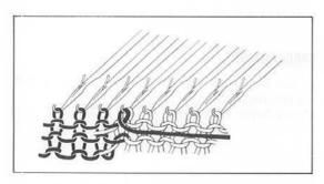
To prevent separation of ground yarn from the contrast yarn at the edge of pattern, wind the contrast yarn around the needle adjacent to the edge needle of the contrast yarn. (To wind the yarn, push the needle to C position, the stitch must remain in front of the latch, and wind the yarn around the needle. Return the needle to B position.)
