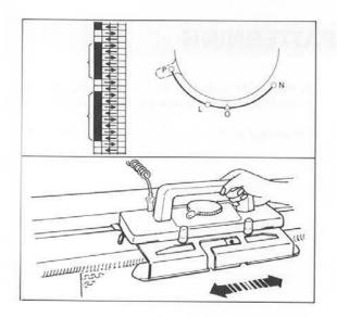
For the pattern rows corresponding with the black marks in the Notation Column, move the Carriage back and forth with the Cam Lever set at "P", and without yarn in the Yarn Feeder.
