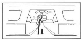
Open the Yarn Feeder and remove the yarn.
