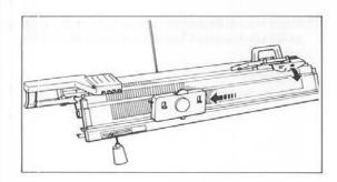
6. Disconnect Ribber Carriage from Arm and move it to the side of Yarn Changer, tilting it towards you.
