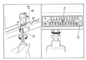
9. Insert Swing Handle shaft "N" into Swing Bearing "O" at the back of the left side of Ribber.
