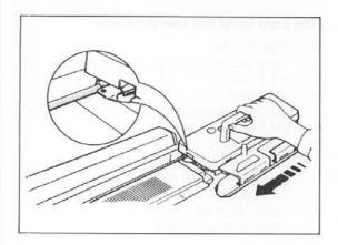
Switch "OFF" the machine, disconnect the Curl Cord from the standard Carriage. Remove the standard Carriage from the needle bed. Take out the Lace Carriage with Lace Arm attached from the Box, raise the Handle and set it on the Needle Bed as shown.
