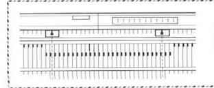
If the edge stitches knit incorrectly, set the Point Cams to exclude two edge needles on both sides, from the pattern knitting area.
