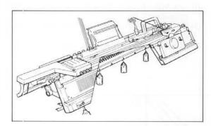
8. Re-set Cam Lever to "O" (STOCKINET) and knit the initial row from the left to the right.
