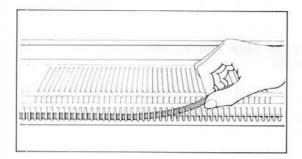
Remove the Close Knit Bar from the Knitter Needle Bed if it is in USP.
