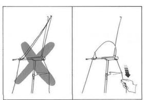
Pull the yarn down through the Yarn Feeder, and guide it under the Arm and over the needles in  ${\sf D}$  position.
