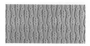
Using the same pattern with the same settings in the same operation, but in different needle arrangement, you can knit different effect on the fabric.
