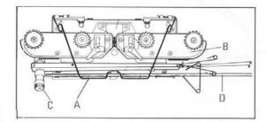
Release the Wire Spring "A", and take out the Arm "B", Auto-Tension "C" and Yarn Rod "D".
