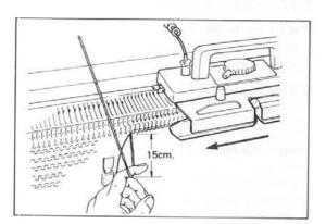
The yarn removed from the Yarn Feeder must be held away from the Arm to prevent it becoming tangled.
