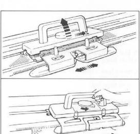
Replace the yarn into the Yarn Feeder, or if the Carriage is at the side opposite the yarn, pass it to the side with the yarn following the instruction given for each type of knitting.
