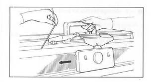
(4) Move Carriage from right to left till yarn goes into Yarn Feeder.
