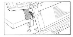
8. Raise both Push-up Cams in arrowed direction.
