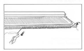
Release the end of the Ravel Cord from the Yarn Clip, and pull it out from the other end.
