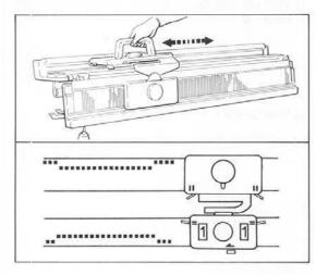
(2) Move Carriage 2 — 3 times carefully across needles in D position and leave it at right side. (Needles in D position will be aligned in B position on both beds.)
