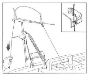
On marked rows, the Carriage transfers stitches only, and does not knit.
