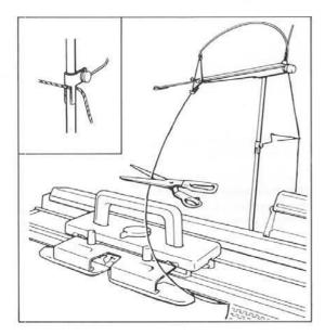
Cut the yarn above the Yarn Feeder, and place the top end in the clip on the Yarn Rod.  $\,$
