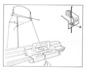
Thread the yarn through the Auto-Tension and into the Yarn Feeder.
