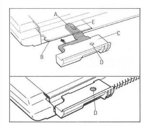
2. Insert finger "A" of Auxiliary Piece into underneath the front edge "B" of Knitter Bed and push backward until plastic part "C" of Auxiliary Piece covers front edge of Bed. (Finger "A" is under the needle bed, part "C" is on top of the needle bed.)
