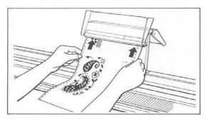
Insert the top end of a Pattern Card into the Card Stand.
