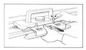
If the yarn has entangled with the Brushes on the Arm or Yarn Feeder, remove the Arm from the Carriage and disentangle the yarn.
