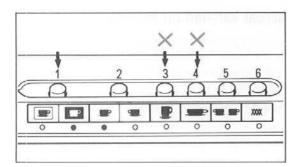
To prevent the end stitches from knitting incorrectly, set the Point Cams to exclude the edge needle from the pattern knitting area.
