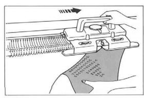
Set the Cam Lever to "0" (STOCKINET) and move the Carriage across the fabric.
