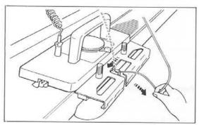
When the black mark in the Notation Column shows above the Card Slot, remove the yarn from the Yarn Feeder.
