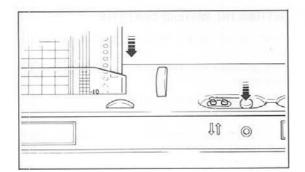
Push the Inspection Button "OFF". (Light is off and the Card is fed by 10 rows downwards and the pattern on the first row is memorized. While memorizing the pattern, you will hear a scanning sound.)
