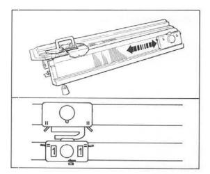
. Disconnect Ribber Carriage and move it twice accross the needles to drop stitches on Ribber needles.
