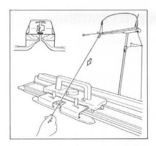
Open the Yarn Feeder Gate, and take the yarn from the Yarn Clip, and pull it down to the Yarn Feeder.
