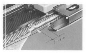
During knitting, make sure the Carriage clears the Separator by  $2\,-\!-\!3\mathrm{cms}$ .
