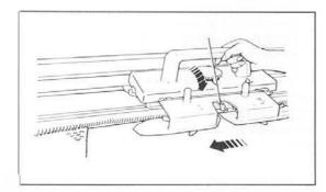
With the top of the Carriage up, pass the Carriage to the side with the yarn end. Press down the top of the Carriage and continue to knit.
