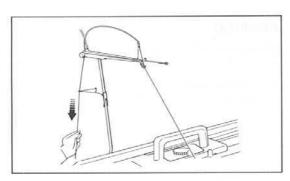
Take up the slack by pulling the yarn back from behind the Yarn Rod till the Tension Spring is almost horizontal.
