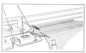
Push the first needle to D position for stockinet (or C position in partial knitting) and move the Carriage to the other side of the needle bed.
