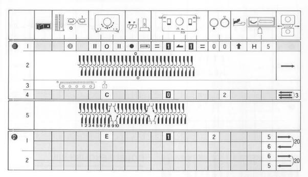
Note: Swing Ribber by 2 pitches for K1.P1. rib and 1 pitch for double rib.
