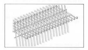
3. Using the straight edge of Needle Pusher push the same number of needles on Knitter and Ribber to D position.
