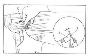
6. Push Ribber on both sides against Knitter until there is no gap between Ribber Stopper "I" and Auxiliary Piece "J".
