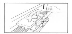
To correct the irregular zigzag yarn, pull down the yarn from the Tension-Spring toward the Yarn Feeder.
