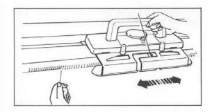
Pulling down the Ravel Cord tightly, move the Carriage slowly to the other side, passed the end needle by  $2-\!\!\!\!-3\text{cm}.$  Then continue to move the Carriage to and fro several times.
