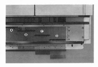
The letters A, B, C and D associated with brackets "]" are engraved at the both ends of the needle bed. The needles covered by each bracket function as below.
