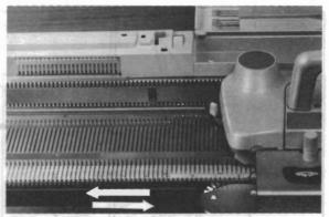
\* Move the Carriage slowly from side to side across the Needle Bed to line the needles in B position, leaving it on the right side of the needle bed.
