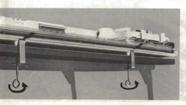
(4) Insert the Clamps into the slots at the bottom of the casement. Fasten the Clamps by tightening screws.
