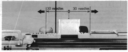
(3) Do not pull the Carriage off the Needle Bed.
