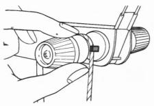
\* Be sure that the yarn is threaded under the copper coloured Guide Pin.
