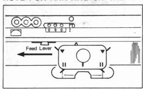
\* Move the Carriage till it hits the Feed Lever located at the Row Counter so as to feed the Pattern Paper.
