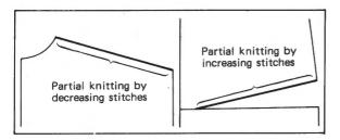
Partial knitting is a practical method for shaping a gentle slope, such as a shoulder, back of slacks and so on, by decreasing or increasing stitches.
