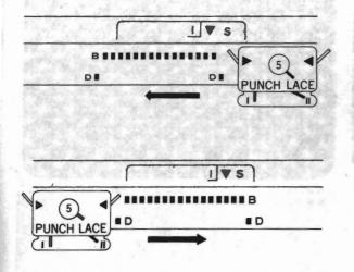
(5) When moving the Carriage from right to left, be sure to push up the end one needle on both sides to D position every time and knit.
