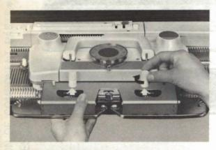
(3) Loosen the Carriage Arm Nuts and slide the Carriage Arm under the Nuts as far as it goes and firmly tighten the Nuts.
