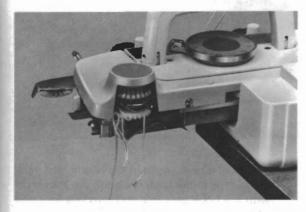
(1) If the yarn is entangled on the gear wheel of the "Memory Bank" move the Carriage to the side of the Knitter as illustrated.
