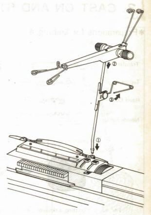
(2) The Yarn Rod can be installed on either side of the Case Handle. An optional Auto Tension can be used together for knitting with four differentcolour yarns.
