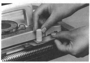
(4) Replace the Carriage Fastener to lock the Carriage securely.
