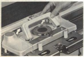
(4) Raise the Carriage Handle until it stands in a locked position.
