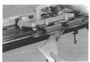
Open the Yarn Feeder Gate and pull yarn out from the Yarn Feeder. Set the Cam Lever to STOCKINET and move the Carriage across once. The fabric will come off of the needles.
