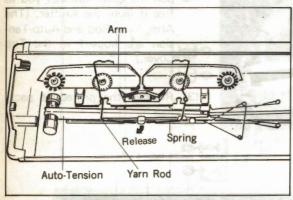
(2) Release the wire spring which secures, inside the top cover, the Yarn Rod, Auto-Tension and Carriage Arm. Remove the Arm from the cover.
