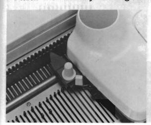
\* When knitting with the tension gauge of 30 rows using thick yarn, the Pattern Paper is fed only half the lenth of a stitch size per row. Therefore, the Auxiliary Feeding Cam should be attached to the left side of the Carriage to feed it double the length per row.
