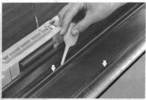
(2) Apply lubricant to a clean cloth, wipe with the oiled cloth across the Needle Bed rail and the needle butts from left to right and right to left. Remember, excessive oil is not required.
