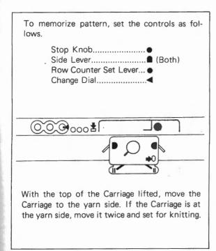
Note:\* In case of pattern knitting with the Stop Knob at •, repair as in the stockinet. This Knitter memorizes the pattern on the Punch Card on the preceding row in the rear Memory Bank. When the Carriage is moving back, the pattern memorized in the Memory Bank will be knitted and at the same time, the rear Memory Bank memorize the pattern on the Punch Card to be knitted on the next row. Therefore, if erroneously knitted, work as follows:—
