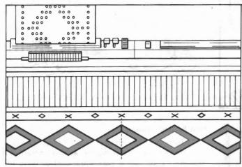
\* On the Needle Bed are X and \$\ighthereo\$ marks and also needle number mark. Pattern is knitted over X and \$\ighthereo\$ mark repeatedly.
