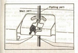
(3) After the platting yarn has been threaded correctly, as shown in the diagram, thread the main yarn through Yarn Feeder ①. Close the Yarn Feeder Gate and start knitting.
