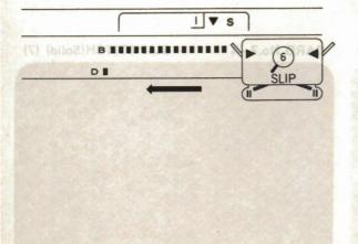
Slip stitch patterns are formed by the yarns crossing at the back of the loops which were not knitted and pulled up by needle selection.
