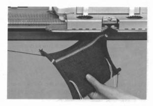
(9) Unthread the yarn from the Yarn Feeder, setting the Cam Lever to STOCKINET, move the Carriage once, and the fabric will come off the needles.
