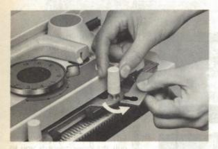
(1) Loosen the right Arm Nut and remove the Carriage Fastener. (Be very careful not to lose the Carriage Fastener, as this is used for securing the Carriage to the Needle Bed when the Knitter is stored or handled.)
