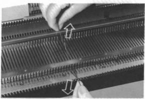
(3) Bring the damaged needle to D position. Close the latch and push the hook downward. The shank will come out of the Needle Bed. Pull the needle out of the Needle Bed lifting the shank upward. If the needle is removed in the middle of the Needle Bed, it will hit the Center Panel. In this case, pull the shank firmly upward, then pull the needle from the Bed.
