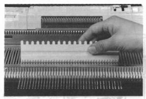
\* Using the smooth side of the Needle Pusher, bring the required number of needles to D position on both sides of the centre 0 mark on the needle bed.
