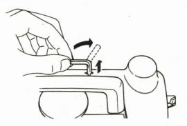
Install the Accessory Box Cover at the right end of the machine by fitting its opening to the stud. You can use this Cover as an useful tray while knitting.
