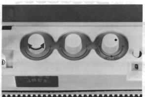
(2) Next, adjust the number of gauge rows to the pointer in red in the row number window, by turning the Row Number Dial. The row numbers are indicated in two sections. Be sure to read the section corresponding to the 30—60 or 61—120 rows depending on the gauge rows counted on your swatch.
