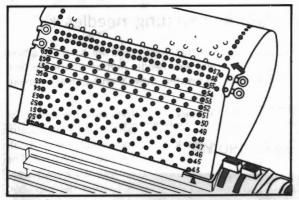
(3) Overlap the ends of the Card, with the end of your side on top of the other as illustrated and line up the two holes on each side. Insert the Card Snaps and join the ends.
