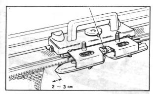
Move the Carriage at an even speed ensuring it has passed the last knitted needle by 2-3cm, before changing direction.
