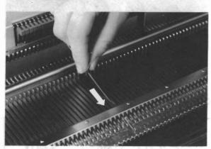
(4) To install a new needle in the Needle Bed, hold the butt with the latch open and slip the needle with the hook part first and reversing the order of the previous paragraph (3).
