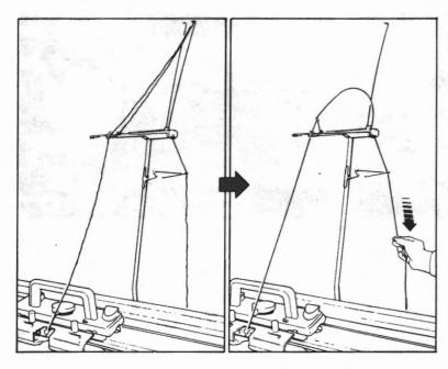
Incorrect threading of the yarn through the Auto-Tension will never assure success in knitting. Before starting to knit, make sure of the following.
