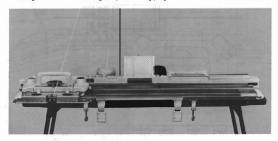
(2) When moving the Carriage, ensure at all times that the Carriage has passed the centre portion of the Needle Bed (about 30 needles on both sides of the centre 0 mark). The Carriage must always be moved at an even speed.
