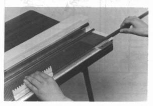
(5) Replace the Needle Retainer. If it hits against the needles, push the needles down as illustrated. Push the Needle Retainer toward the edge of the Needle Bed so it will not go in crooked.
