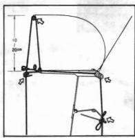
Is yarn correctly guided through \* Does yarn come out smoothly. the Auto-Tension?
