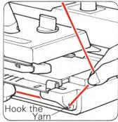
Take Yarn 1 out of Yarn Feeder "A". If you slide the K-Carriage slightly to the right the yarn can be removed easily.
