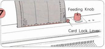
Turn the Feeding Knob and rotate the Card to the starting line. Set the Card Lock Lever to the "O" mark.
