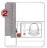
Insert the Punch Card and rotate it to Starting Line.
