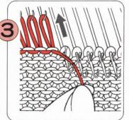
Hang the Cast-on Thread over the hooks of the needles in E position, and knit them back to A position by hand.
