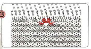
Loop the yarn around the two needles by hand as shown above.
