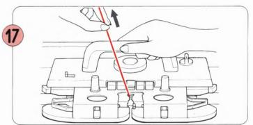
Continue knitting with the K-Carriage, pulling the yarn slightly on the first row to remove any slackness.
