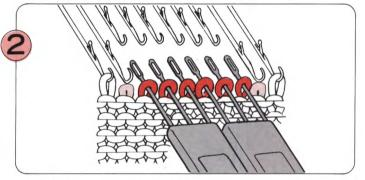
Transfer 3 stitches onto both 3-eyed Transfer Tools as shown.
