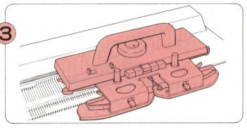
Move the K-Carriage across the needlebed a few times to align the needles, ending with the K-Carriage on the right.
