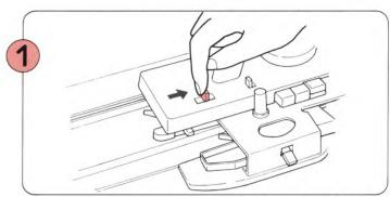
Set the Holding Cam Lever to H and the Cam Buttons and Change Knob according to the pattern.
