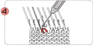
Lift the Transfer Tool slightly so that the stitch slides off into the hook of the needle. Then remove the Transfer Tool. One stitch has been transferred.
