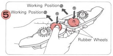
Remove the Sinker Plate Assembly from the K-Carriage and turn it over; Put the Rubber Wheels into working position @ as shown. Attach the Sinker Plate Assembly back on the K-Carriage again.
