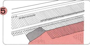
Waste knit Part (2) and remove this from machine. Return needles to A position.
