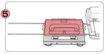
Place the L-Carriage securely on the Extension Rail at the left.
