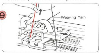
Move the K-Carriage to the right, pulling the main yarn upwards slightly – ensure that the weaving yarn is in the right Weaving Yarn Guide.
