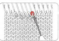
(1) Place the eye of the Transfer Tool into the hook of the needle.
