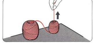
Yarn pulled from the centre of a rewound ball should come out freely without lifting the ball from the table.
