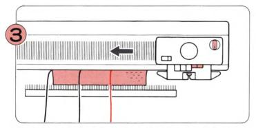
Push in both Part Buttons and move the K-Carriage across to the other side of the needle bed.
