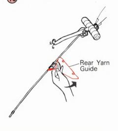
Insert the end of the Rod into the hole at the back of the machine.
