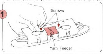
Remove the two screws and the Yarn Feeder from the Sinker Plate Assembly.
