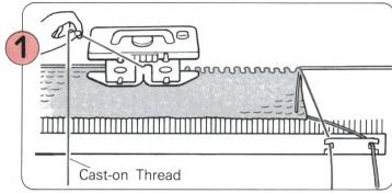
Knit several rows with waste yarn and then knit one row with the Cast-on Thread. (Refer to P.99).
