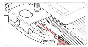
While knitting make sure the contrast yarn goes under the concavity in the Sinker Plate.
