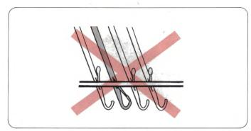
\*When working Intarsia, always make sure the latches are open, otherwise the stitches will drop.
