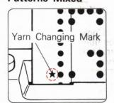
When the Yarn Changing Mark (asterisk) on the leftside of the Punch Card comes to the card opening change the setting of the Card Lock Lever ("▽" or "∇") and continue knitting.
