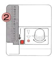
Insert the Punch Card and rotate it to Starting Line. Set the Card Lock Lever at "•" mark.
