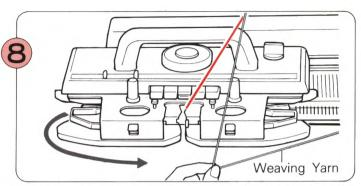
Remove the weaving yarn from the left Weaving Yarn Guide by moving the K-Carriage slightly to the left. Pass the weaving yarn under the K-Carriage to the righthand side.
