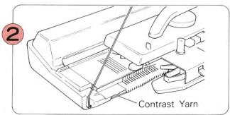
Take the contrast yarn out of Feeder "B" and hook it around the notch at the end of your machine. Then continue knitting with the main yarn only, bringing the end needles back to B position on each row.
