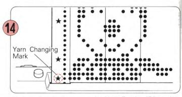
Change the contrast yarn in. Yarn Feeder "B" to the next one when the Yarn Changing Mark (asterisk) on the left side of the Punch Card comes to the card opening.
