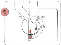
Set the Change Knob to N.L. The Cam Buttons will be released automatically.
