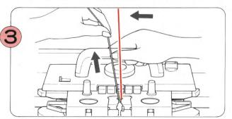
When the needles are selected across the row again for the pattern, rethread the contrast yarn into Feeder "B" and knit the row, holding the contrast yarn as shown so that no loops form at the edges.
