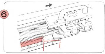
Move the K-Carriage without knitting, to align the needles in D position.
