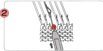
Holding the Transfer Tool in line with the needle, use it to push the needle back so that the stitch slips onto the Transfer Tool.
