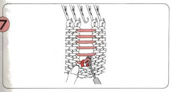
The latch closes with this new stitch in the hook. Gently slip the old stitch off the end of the Latchet Tool. A purl stitch has been formed.
