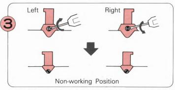
Cancel the working of end needle selection mechanism. (Refer to P.22).
