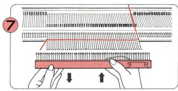
(1) Take the Cast-on Comb out of the Case and choose the length according to the number of needles. (Refer to P.20).
