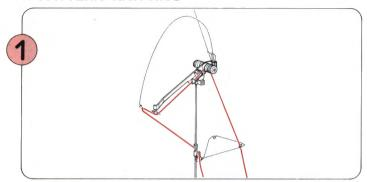
Thread the main yarn into the righthand Yarn Tension Unit.
