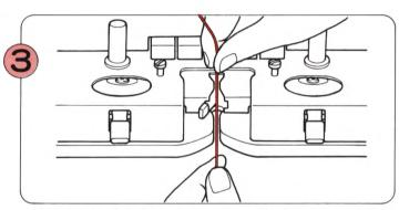
Thread the yarn into Yarn Feeder "A".
