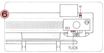
Push both Tuck Buttons at the same time. Set the Card Lock Lever at "-w-" mark.
