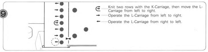
Use either the L-Carriage or the K-Carriage according to the mark on the left side of the Punch Card.
