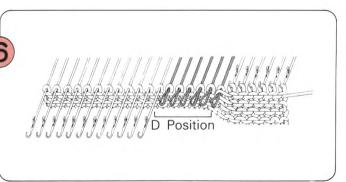
Manually push the needles to be increased from E to D position.
