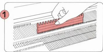
Place the K-Carriage at the right. Using the flat side of the 1/1 Needle Pusher bring the needles forward to E position.
