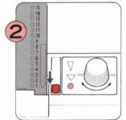
Insert the Punch Card and rotate it to Starting Line. Set the Card Lock Lever at "o" mark.
