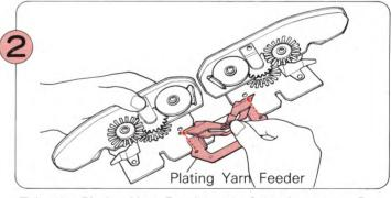
Take the Plating Yarn Feeder out of the Accessory Box and fit it into the Sinker Plate Assembly as shown above.
