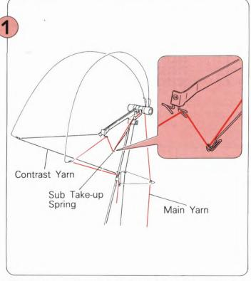
Thread the main yarn into the righthand Yarn Tension Unit including Sub Take-up Spring and the very fine contrast yarn into the lefthand one.
