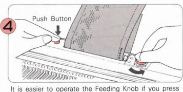
It is easier to operate the Feeding Knob if you press down on the Push Button at the same time.
