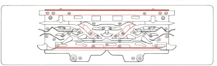
Should the K-Carriage feel heavy to operate, you should clean and lubricate the areas indicated above, using an oily cloth.
