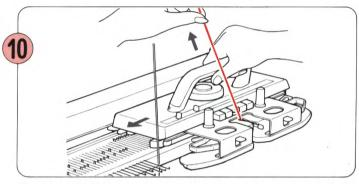
Continue knitting at the same time placing the weaving yarn into the left or right Weaving Yarn Guide according to the direction of the K-Carriage, and pulling the main yarn upwards slightly.
