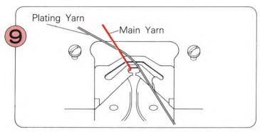
Pass the end of the plating yarn behind the main yarn.
