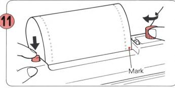
Wind the Punch Card back to the mark you made on it. (Leave the Card Lock Lever as it is " $\nabla$ ").
