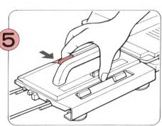
Push the Release Button and place the L-Carriage securely on the left Extension Rail.
