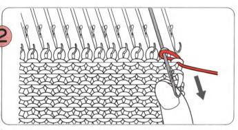
Bring this needle forward so that the two stitches are behind the latch.
