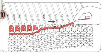
Pull the yarn sideways slightly so that it becomes tight in the needle hooks.
