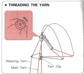
Thread the main yarn into the righthand Yarn Tension Unit and the weaving yarn into the lefthand one. Adjust the Tension Disc as shown according to the weaving yarn.
