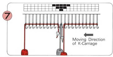
Beginning at the side nearest to the K-Carriage, and working away from the K-Carriage, lay the yarns in the open needle hooks as illustrated.
