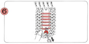
Catch the next horizontal bar above with the hook of the Latchet Tool. Pull the Latchet Tool towards you.
