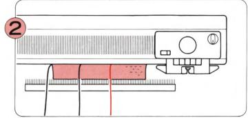
If the K-Carriage is at the same side of the knitting as the yarn, remove the K-Carriage from the needlebed and place it at the opposite side.
