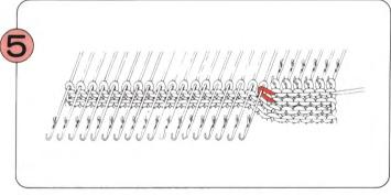
The yarn is wrapped around the end needle in Holding Position as shown above.
