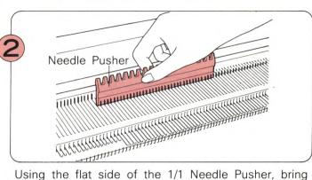
Using the flat side of the 1/1 Needle Pusher, bring forward 60 needles to B position (30 needles on either side of the centre mark"0").
