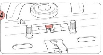
Push the Cam Buttons according to the pattern.
