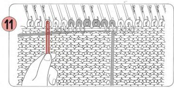
Fold the separate piece of finishing yarn in half and place it over the needle adjacent to the last selected needle at the left.
