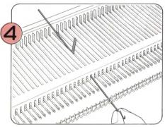
Press down at the hook end so that the shank end of the needle is raised clear of the needle bed.
