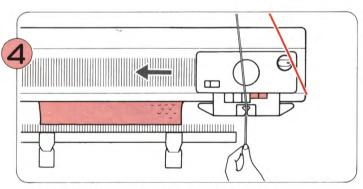
Thread Yarn 2 into Yarn Feeder "A" and knit two rows.
