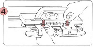
After you have changed the Yarn Feeder, screw the Sinker Plate Assembly back on the K-Carriage.
