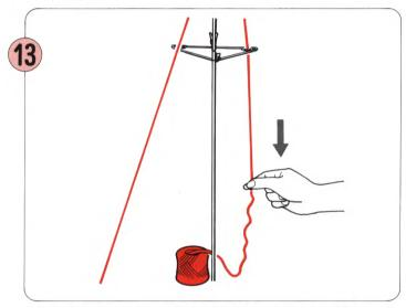
Pull down the loose unravelled yarn from behind the Rear Yarn Guide.
