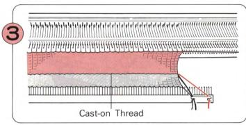
Knit several rows with waste yarn, then one row with the Cast-on Thread. With main yarn, working in stocking stitch, knit the number of rows required for double the length of the hem.
