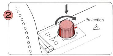
Press down on the Feeding Knob and turn it one hundred and eighty degrees in a clockwise direction. The card will feed back seven rows, and you can see the pattern perforations for the actual row you are knitting.
