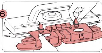
Screw the Sinker Plate Assembly back onto the K-Carriage.
