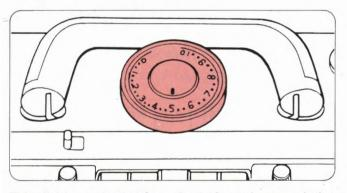
This dial is graduated from 0 to 10, each space being subdivided into three parts. With this dial you can alter the size and tension of your stitches. 0 is the tightest tension (i.e. the smallest stitch) and 10 is the loosest tension (i.e. the largest stitch). You should adjust the dial to a higher or lower number according to the thickness and type of yarn you are using.
