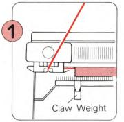
Knit a few rows in stocking stitch and place the K-Carriage on the left side of the machine. Hang the Claw Weights evenly along the Cast-on Comb.
