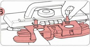
Place the K-Carriage onto either of the Extension Rails. Screw the Sinker Plate Assembly back onto the K-Carriage.
