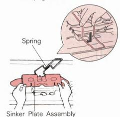
Screw the Sinker Plate Assembly onto the K-Carriage.
