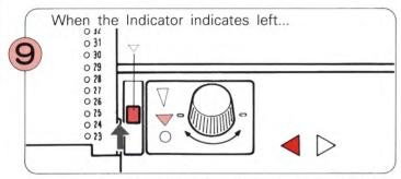
When the Carriage Direction Indicator indicates left, set the Card Lock Lever at "\( \neq \)" mark. Move the L-Carriage from left to right and continue knitting.
