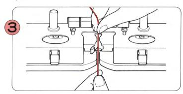
Thread the main yarn into Yarn Feeder "A".
