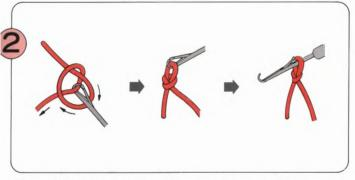
Thread the yarn into the Yarn Tension Unit. Now make a chain stitch using the Latchet Tool as shown.
