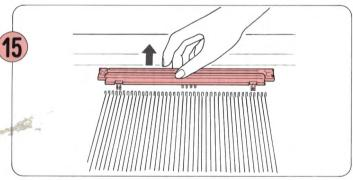
Remove the One-point Cam (or Motif Knitting Cams).
