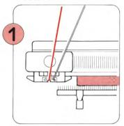
Knit a few rows in plating and place the K-Carriage on the left side of the machine. Hang the Claw Weights evenly along the Cast-on Comb. (Refer to P.59-60).
