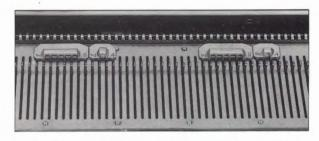
The L-point Cams cannot be used for Fairisle Motif Pattern or Thread Lace Motif Pattern. Remove the L-point Cams after finishing the Isolated Lace Pattern.
