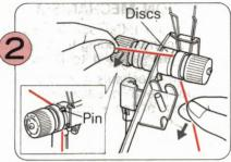
Pass the yarn under the Pin and between the two Discs from behind. Hold the yarn as shown above, and pull it towards you so that the yarn goes under the Pin.
