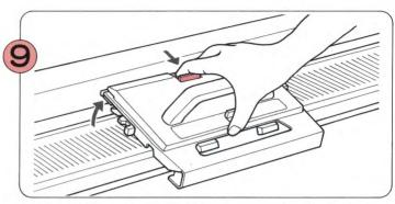
Remove the L-Carriage from the machine by depressing the Release Button.
