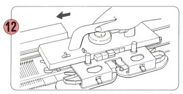
Move the K-Carriage from right to left without yarn. The needles are selected according to the pattern row.
