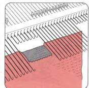
Waste knit the stitches for Part (1) only and return needles to A position.
