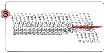
Knit one row. The needles in B position (B and D position in the case of pattern knitting) have been knitted and those in E position have not been knitted.
