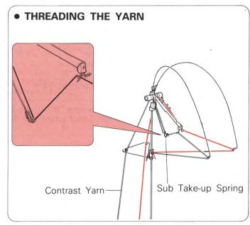
Thread the main yarn into the righthand Yarn Tension Unit, and the contrast yarn into the left Yarn Tension Unit, including the Sub Take-up Spring.
