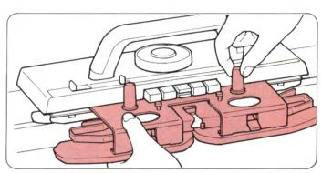
• Is the Sinker Plate Assembly joined correctly to the K-Carriage?
