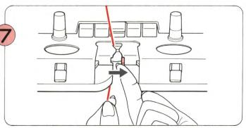
Keeping hold of the end of the yarn with your left hand, close the Yarn Feeder Lever.
