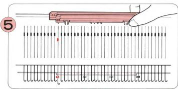
Place the One-point Cam on the needle bed by matching the
