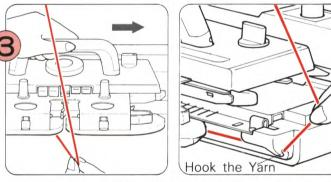
Take Yarn 1 out of Yarn Feeder "A". If you slide the K-Carriage slightly to the right the yarn can be removed easily.
