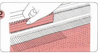
Using the flat side of the 1 x 1 Needle Pusher, bring the needles for Parts (2) and (3) forward to E position.
