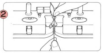
Thread the waste yarn into Yarn Feeder "A".
