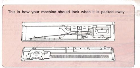
Fold down the handle on the L-Carriage. Push the Release Button and replace the L-Carriage in the Carrying Case.
