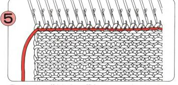
The casting off (binding off) is now completed and you can remove the knitting from the machine.
