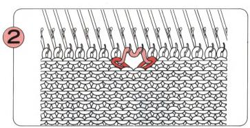
Place empty needles in B position and knit one row. The yarn has hooked over these two needles.
