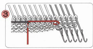
Wrap the yarn under the stem of the first needle in E position as shown, then lay the yarns for the Intarsia pattern. Knit one row.
