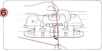
Thread Yarn 1 into Yarn Feeder "A" and knit two rows. Change the Yarn in the Yarn Feeder "A" every two rows.
