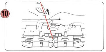
Move the K-Carriage to the left, holding the yarn as shown so that no loops are formed.
