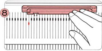
Place the One-point Cam (or Motif Knitting Cams) on the needles where you want the pattern to be. (Refer to P.45).
