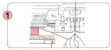
Remove the Claw Weights and take the yarn out of Yarn Feeder.
