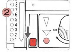
Set the Card Lock Lever at "o" mark. Take the contrast yarn out of Yarn Feeder "B"
