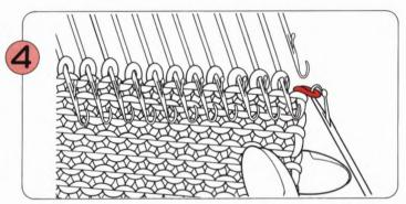
Beginning at the righthand edge, hook the first stitch onto the Latchet Tool.
