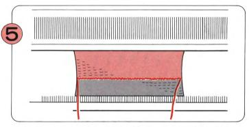
One row has been knitted with the Cast-on Thread and this separates the waste knitting from the main knitting.
