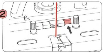
Place the K-Carriage on the right of the machine and push in the right Part Button.
