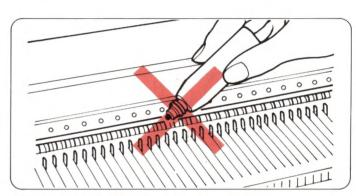
Do not put oil directly onto the machine.
