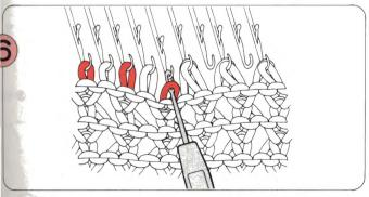
Return any stitches that have been transferred back onto the adjacent needles using the Transfer Tool.
