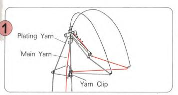
Thread the yarns into the Yarn Tension Unit as shown.
