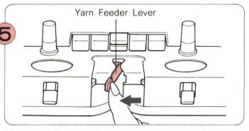
Open Yarn Feeder A by pushing the Yarn Feeder Lever to the left.
