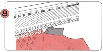
Knit Part (2) ending with waste knitting and remove this from machine. Return needles to A position.
