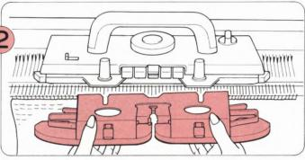
Loosen the knobs and remove the Sinker Plate Assembly
