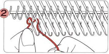
Beginning at the left, and working from left to right, wind the yarn around the needles in an anticlockwise direction. Do not wind the yarn too tight.
