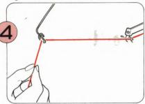
Thread the yarn into the eyelet of the Take-up Spring.
