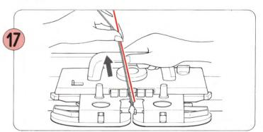
Continue knitting with the K-Carriage, pulling the yarn slightly on the first row to remove any slackness. \*Put the Row Counter and Knit Leader Tripper back in operation.
