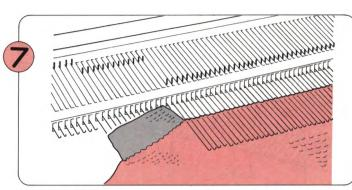
Waste knit Part (2) and remove this from machine. Return needles to A position.
