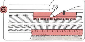
Starting with the second needle from either end, bring every alternate needle forward to D position using the 1/1 Needle Pusher. The end needles must remain in B position.
