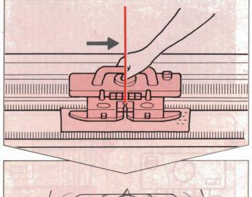
**2** Move the K-Carriage slowly to the right (to the left in Double Length Pattern). The needles are selected to B and D positions.
