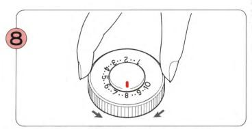
Set the Tension Dial according to the yarn you are using.
