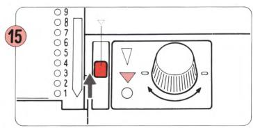
Set the Card Lock Lever at " $\neg$ " mark. (When working in Double Length Pattern, set it at " $\forall$ " mark.)
