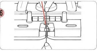
Thread up the yarn into Yarn Feeder.
