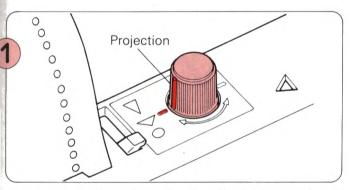
Set the projection of the Feeding Knob at - mark on the Panel without pushing it.
