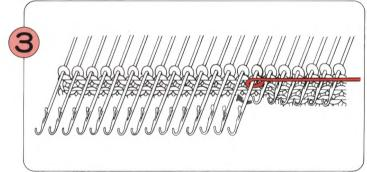
Wrap the yarn under the stem of the first needle in E position as shown, then lay the yarns for the Intarsia pattern. Knit one row.
