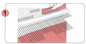
Bring the two sets of needles for Part (2) into E position.
