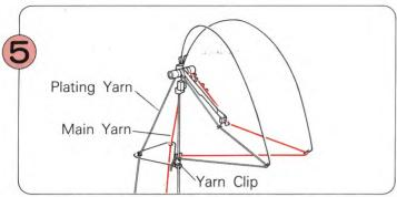
Thread the yarns into the Yarn Tension Unit as shown.
