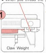
Knit a few rows in stocking stitch and place the K-Carriage on the right side of the machine. Hang the Claw Weights evenly along the Cast-on Comb.
