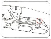
If you want to knit multi-colour rib pattern, connect the Latch Opening Plate to the connecting arm assembly.
