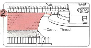
Working in stocking stitch, knit the number of rows required for double the depth of the hem (e.g. if hem is to be folded under 2.5 cms (1") then knit 5 cms (2").
