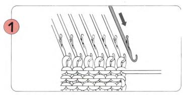
On the K-Carriage side, bring one edge needle forward from A to B position.
