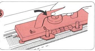
Lift up the K-Carriage towards you to remove it. Place it onto either of the Extension Rails. Set the Change Knob to N.L.
