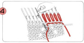
On the K-Carriage side, manually knit the next needles back to A position using the Cast-on Thread.
