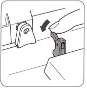
Set the Row Counter to 000 and the Row counter Tripper to working position.
