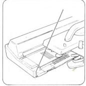
Take Yarn 2 out of Yarn Feeder "A" and hook Yarn 2 around the notch at the end of your machine. \*Hook Yarn 1 around the notch at the right end of your machine and Yarn 2 around the notch at the left end.
