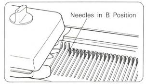
Make sure the K-Carriage (or the L-Carriage) clears the knitting before you move it back in the other direction. You will hear a "Click" at the end of a row.
