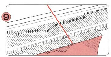
Using your Transfer Tool, replace any stitches that are on the stems of the needles back into the hooks, so that they will not drop off. (The following steps illustrate this technique).
