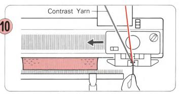
Thread the contrast yarn into Yarn Feeder "B" – there is no need to open the Yarn Feeder Lever when you do so.
