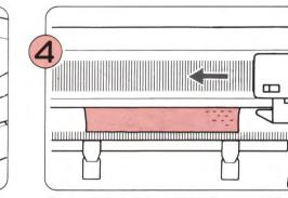
Thread Yarn 2 into Yarn Feeder "A" and knit two rows. Change the Yarn in Yarn Feeder "A" every two rows. (When you change the yarns, take care not to cross them over each other.)
