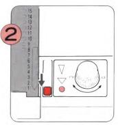
Insert the Punch Card and rotate it to Starting Line. Set the Card Lock Lever at "O" mark.
