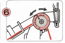
Set the arrow mark according to the thickness of the yarn.
