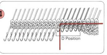
Bring the needles to be increased from E to D position and lay the yarns for the Intarsia pattern. Knit one row.
