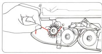
Remove the K and L Carriages from the needle bed and brush away any dust or fluff. Check that the brushes are free from fluff or strands of yarn, and that they revolve smoothly.
