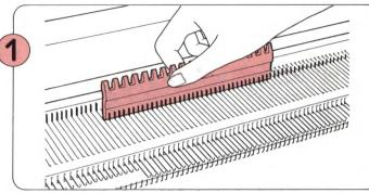
Using the flat side of the 1/1 Needle Pusher, bring forward the required number of needles to B position.
