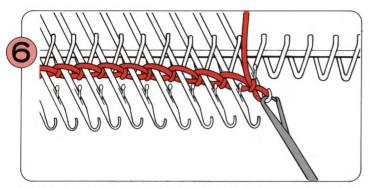
When you get to the last needle, transfer the loop from the Latchet Tool into the needle hook.
