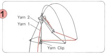
Thread Yarn 1 into the righthand Yarn Tension Unit and Yarn 2 into the lefthand one. Follow the steps 1-6 on P.34.
