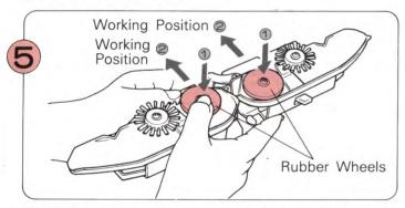
Remove the Sinker Plate Assembly from the K-Carriage and turn it over. Put the Rubber Wheels into working position ② as shown. Attach the Sinker Plate Assembly back on the K-Carriage again.
