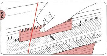
After unravelling a row check that all the stitches are in the needle hooks. Using the flat side of the 1/1 Needle Pusher, align the needles in B position.
