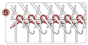
Pull the yarn through the edge hook. Hang the Cast-on Comb over the loops and gently pull it downwards.
