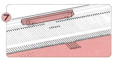
Move the K-Carriage from left to right. The needles corresponding to the One-point Cam are selected in pattern.
