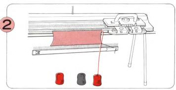
Take the yarn out of the Yarn Feeder and the Yarn Tension Unit. Prepare the other balls of yarn, and place them on the floor at your feet.
