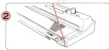
Secure the yarn by hooking it into the slot at the edge of your machine.
