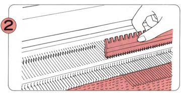
Using the flat side of the  $1 \times 1$  Needle Pusher, bring the needles for Parts (2) and (3) forward to E position. These needles will not knit.
