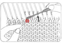
(4) Transfer the stitch into the hook of the needle.
