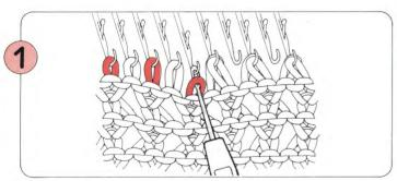
Set the Card Lock Lever at "o" mark. Return any transferred stitches to the adjacent needles and put all needles in B position.
