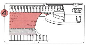
Knit half the depth of the hem (e.g. to what will be the foldline). Place the K-Carriage on the Extension Rail at the right. Note the number showing on the Row Counter.
