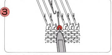
Lift the Transfer Tool together with the stitch, and place it onto the adjacent needle.
