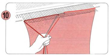
Lay the yarns and knit the third row. Continue knitting in this way, laying your yarns according to your pattern chart. (Repeat Steps <a>(9-60)</a>).
