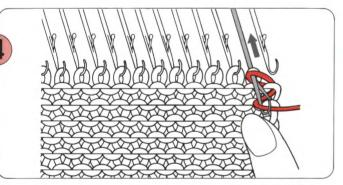
Manually push the needle back so that a single stitch is formed.
