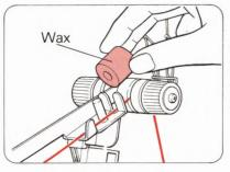
When you start to knit, place the Wax which you will find in the Accessory Box on the Wax Stand. The Wax helps the yarn to slide smoothly.
