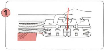
Knit the final row from right to left. Loosen the Tension Dial for this row (e.g. if main tension is say 4-6, knit the final row at tension 9-10).
