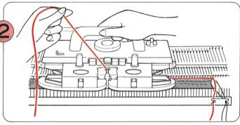
Thread the Cast-on Thread into Yarn Feeder "A". Hold the end as shown and knit one row. Remove Cast-on Thread from Yarn Feeder "A".
