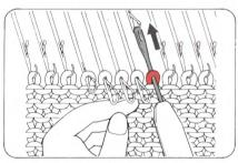
(3) Push the Transfer Tool away from you towards the machine until the stitch is on the Transfer Tool.
