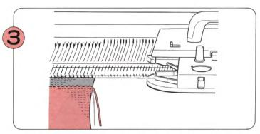
After knitting several rows with waste yarn, remove the knitting by passing the empty carriage across the stitches.
