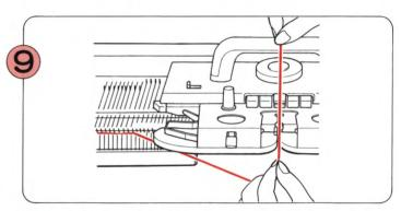
Thread the yarn into Yarn Feeder "A". (Refer to Steps \$-\$\mathcal{O}\$ on P.25).
