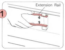
Remove the Extension Rails from the Carrying Case.
