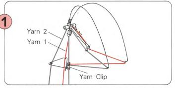
Thread Yarn 1 into the righthand Yarn Tension Unit and Yarn 2 into the lefthand one. Follow the steps 1-0 on P.36.
