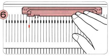
Push the Cam back as far as it will go, placing it in parallel with the Rear Rail. Make sure it is inserted correctly.
