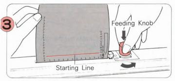
Feed the Punch Card into the opening, making sure that the line on the Card is parallel with the top of the slot.
