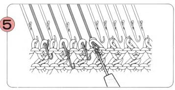
Use the Transfer Tool to replace any stitches on the stems of the needles back into the hooks.
