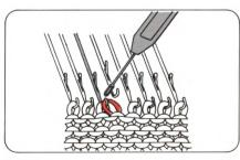
If you need to replace a needle whilst you have knitting on the machine transfer the stitch from the faulty needle onto an adjacent needle. Replace the stitch after you have completed the replacement.
