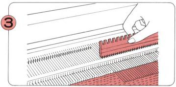
Using the flat side of the  $1 \times 1$  Needle Pusher, bring the needles for Parts (2) and (3) forward to E position. These needles will not knit.
