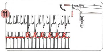
Hook the Cast-on Comb over the loops and let it hang down. Give the Comb a gentle pull downwards.
