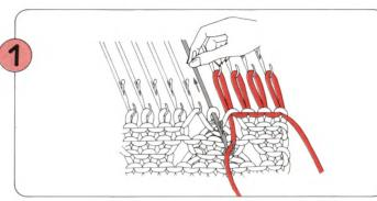
On the opposite side to K-Carriage manually knit the needles you want to decrease back to A position using the Cast-on Thread.
