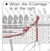
Wrap the finishing yarn around the hook of the needle adjacent to the first selected needle, and pull down gently.
