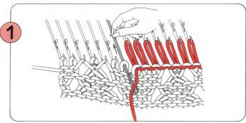
Using the Cast-on Thread, manually knit the needles you want to decrease back to A position.
