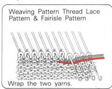
Wrap the yarn by passing it under the stem of the first needle in E position as shown.
