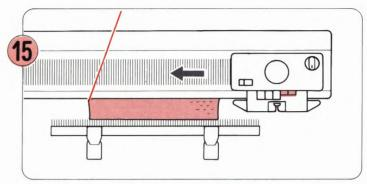
If the yarn is now on the opposite side of the knitting to the K-Carriage, you can move the K-Carriage across the needles without knitting as follows:
