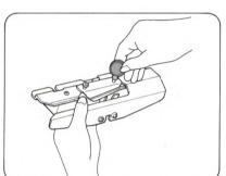
(1) Remove the screw to take out the Yarn Feeder.
