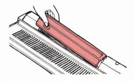
Hold the lid and replace it as shown. When it is in place, lock the two catches on either side of the Handle.
