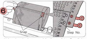
Using the plastic snaps, join the card to allow it to
