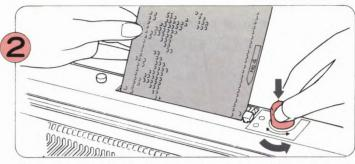
With the number facing you, insert the bottom edge of the Punch Card into the slot. Make sure you hold the Punch Card straight.
