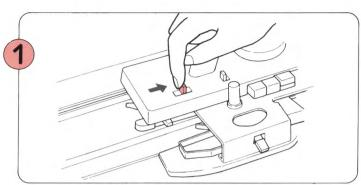
Set the Holding Cam Lever to H and the Cam Buttons and Change Knob according to the pattern.
