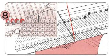
Using your Transfer Tool, replace any stitches that are on the stems of the needles back into the hooks, so that they will not drop off. (Refer to Step 9 (1) – (5) on P.68.)
