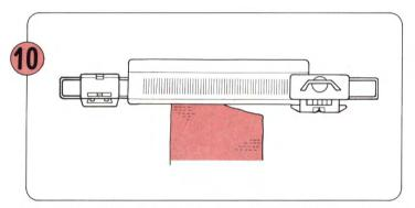
Place the K-Carriage on the right side of the machine and the L-Carriage on the left Extension Rail.
