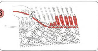
Transfer the first block of stitches in A position back into the hooks of the needles, removing the Cast-on Thread from these, and placing them in B position. Knit one row with the K-Carriage. Repeat Steps ③ – ⑥.
