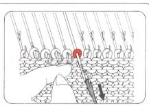
(2) Hold the Transfer Tool in line with the needle and pull it towards you.
