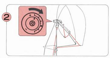
Adjust the Tension Disc to the thickness of the contrast yarn.
