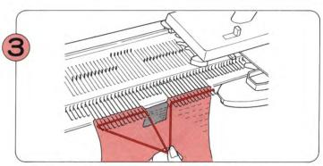
Return the Part (2) needles from E to D position and knit both shoulders according to your pattern.
