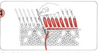
Manually knit the next needle back to A position using the Cast-on Thread.
