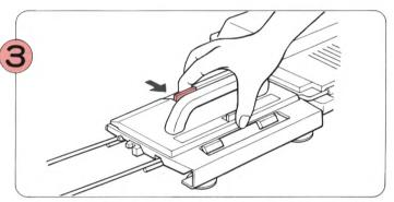
Place the L-Carriage securely on the left Extension Rail using the Release Button.
