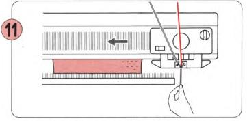
Hold the end of the plating yarn with your lefthand, and move the K-Carriage to the left. Once the needles have caught the yarn, you can release the yarn end. Continue knitting in this way. You are now knitting plating.
