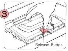
Remove the L-Carriage by pushing the Release Button.
