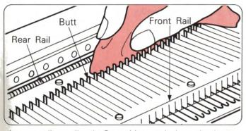
Arrange all needles in B position and clean the butts, rear and front rails as shown, using an oily cloth.
