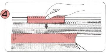
With the flat side of the 1/1 Needle Pusher, bring the needles in A position forward to B position.
