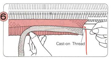
When you have knitted several rows you can pull out the Cast-on Thread. The waste knitting will fall away.
