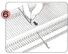
With the latch open, insert the new needle as shown.
