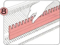
Holding the needles down with your hand or the flat side of your 1/1 Needle Pusher, push the sponge Presser Bar back in place.
