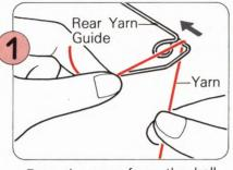
Pass the yarn from the ball through the Rear Yarn Guide sliding the yarn through the eyelet.
