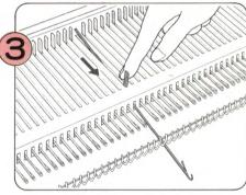
Push the faulty needle forward to E position as far as it will go.
