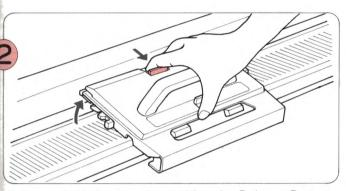
Remove the L-Carriage by pushing the Release Button. If the L-Carriage is caught on the needles, take care when removing it.
