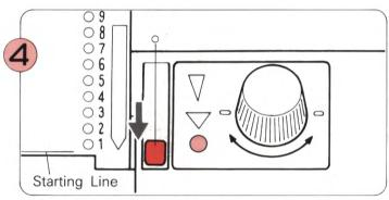
Insert the Punch Card and rotate it to Starting Line. Set the Card Lock Lever at "O" mark.
