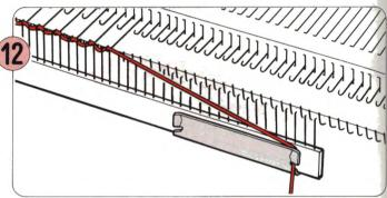
Hook the loose yarn end under the Yarn Clip on the front of the Connecting Plate.
