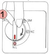
Set the Change Knob to N.L. The Cam Buttons will be released automatically.
