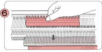
When all the stitches have been picked up, bring the needles forward to E position. Knit one row.
