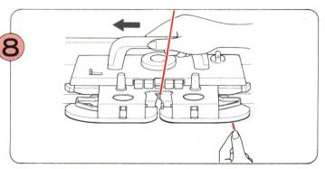
Still holding the yarn end gently, slowly move the K-Carriage to the left. Once you feel the needles catch the yarn, you can release the yarn end.
