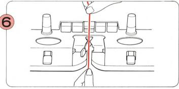
Take the yarn from the Yarn Clip and thread it into Yarn Feeder A.
