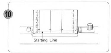
When the last mark below the Starting Line comes to the card opening, one Lace Pattern Card has been completed.
