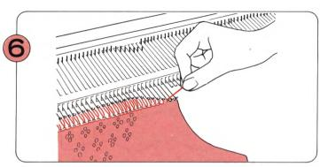
Bring needles from Part (2) from A to B position at the same time replacing the stitches into the needle hooks and removing the Cast-on Thread.
