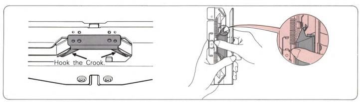
(2) Put the Latch Opening Plate on the Connecting Arm Assembly, and then screw up the Yarn Feeder.
