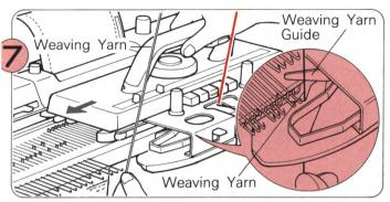
Hold the end of the weaving yarn with your lefthand, and thread it into the Weaving Yarn Guide on the left side of the K-Carriage. Then move the K-Carriage across the needlebed.
