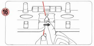
Thread up the yarn into Feeder "A". Put the Row Counter and Knit Leader Tripper back in operation.
