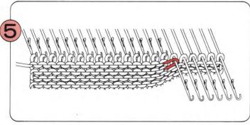
Pull up any loose yarn with your hand and knit one row. The yarn is wrapped around the end needle in Holding Position as shown above.
