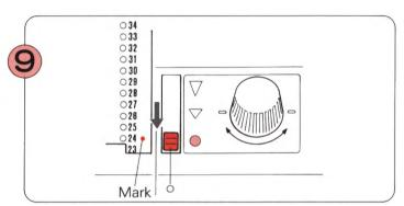
Wind the Punch Card back to the mark you made on it, and set the Card Lock Lever to "o" mark.
