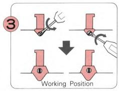
Return End Needle Selection Cams to working position.
