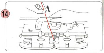
Move the K-Carriage to the right, holding the yarn as shown so that no loops are formed.
