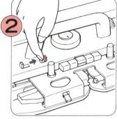
Release the Cam Buttons with the Cam Button Release Lever.
