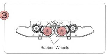
Place the Rubber Wheels in non-working position.
