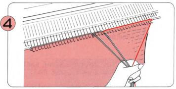
Lay the yarns according to the pattern and continue intarsia knitting.
