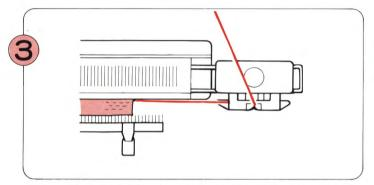
Knit a few rows in stocking stitch and place the K-Carriage on the right Extension Rail. Hang the Claw Weights evenly along the Cast- on Comb.
