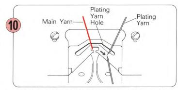
Now thread the Plating yarn into the Plating Yarn Hole. There is an opening at the side and you can pass the yarn through this slit.
