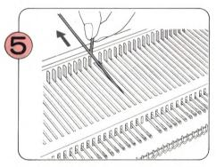
Catch hold of the shank end and lift the faulty needle out from the needle bed.
