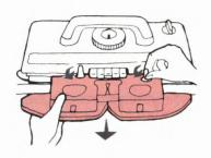
Put the Sinker Plate Assembly in the Case where indicated and secure it with the Spring.
