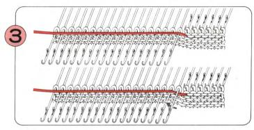
Knit one row. The needles in B position (B and D position in the case of pattern knitting) have been knitted, and the yarn has passed over those in E position. Wrap the yarn under the stem of the first needle in E position. (In the case of pattern knitting, refer to Step @ on P.84).
