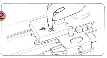
On the K-Carriage, set the Holding Cam Lever to H.
