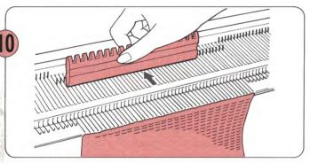
Return the needles to B position using the flat side of the 1/1 Needle Pusher.
