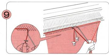
Working in the opposite direction (again away from the K-Carriage) lay the yarns in the open needle hooks for the next row. To avoid a hole appearing where the yarns meet, cross one over the other as illustrated. Now slowly move the K-Carriage across the needlebed.
