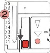
Set the Card Lock Lever at "o" mark. Take the contrast yarn out of Yarn Feeder B.
