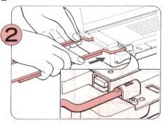
Insert the Extension Rails securely into the holes at both sides of the machine.
