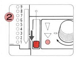
Set the Card Lock Lever at "o" mark. Take the contrast yarn out of the Yarn Feeder "B".
