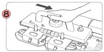
Slide the K-Carriage across onto the needlebed and check it is placed correctly.
