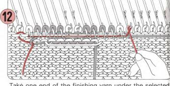
Take one end of the finishing yarn under the selected needles, and wrap it from right to left round the needle adjacent to the last selected needle on the right. (See illustration). Holding the end of the finishing yarn, move the K-Carriage from right to left.
