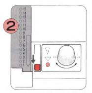
Insert the Punch Card and rotate it to Starting Line. Set the Card Lock Lever at "O" mark.
