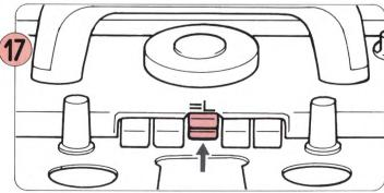
Push both L Buttons (both upper and lower buttons) at the same time and bring back the selected needles to B position.
