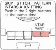
\* Do not operate the K-Carriage if you have depressed both middle Buttons (Upper & Lower) plus either the Tuck Buttons, or the Part Buttons.
