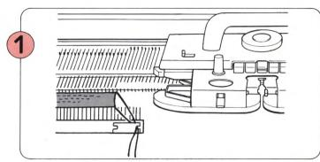
Knit about 10 rows in stocking stitch using waste yarn ending with the K-Carriage at the right of the needle bed. Remove waste yarn from Yarn Feeder and cut the
