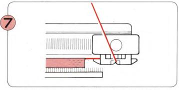
Knit a few rows in stocking stitch, ending with the K-Carriage on the right of the machine.
