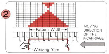
Lay the weaving yarn from the same side as the K-Carriage. Then operate the K-Carriage.
