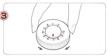
Set the Tension Dial using the Tension Chart on P.48 as a guide.
