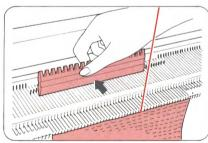
(5) When all stitches are safely in the hooks of the needles, align all needles in B position using the flat edge of the 1/1 Pusher.
