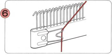
Hook the loose yarn end under the yarn Clip from the front.
