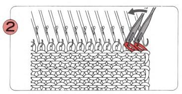
Place the Transfer Tool onto the hooks of the adjacent inside needles, and transfer the stitches.
