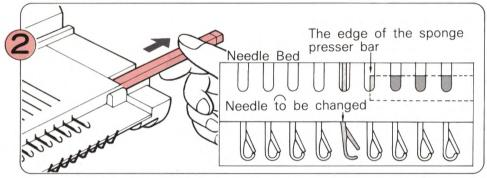
Draw the Bar out by hand until it passes the needle to be replaced.
