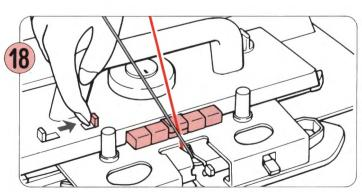
Slide the Cam Button Release Lever to the right to release the Cam Buttons.
