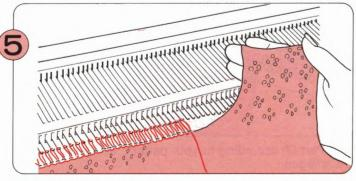
Knit Part (1) according to your pattern using both L and K-Carriages, and return empty needles to A position.
