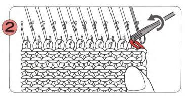
Place the Transfer Tool onto the hook of the adjacent inside needle, and transfer the stitch.
