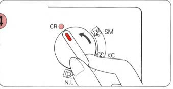
Set the Change Knob to CR to release the K-Carriage from the machine.
