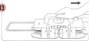
Move the K-Carriage across the needle bed to the same side as the yarn. The needles are selected for the pattern.
