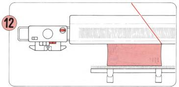
Place the K-Carriage at the opposite end of the needlebed to the yarn. (If the yarn is on the same side as the K-Carriage, refer to P.69 for how to pass the carriage across the needles without knitting). Push both Part Buttons and set the Change Knob to KC or SM.
