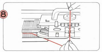
Thread the yarn into Yarn Feeder "A" (Refer to Steps (5) on P.25).
