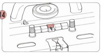
Push the Cam Buttons according to pattern. Thread up the yarn into Yarn Feeder. (If you are using contrast yarn, plating yarn or weaving yarn, don't forget to thread this up.)
