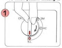
Set the Change Knob to N.L. The Cam Button will be automatically released.
