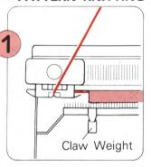
Knit a few rows in stocking stitch and place the K-Carriage on the left side of the machine. Hang the Claw Weights evenly along the Cast-on Comb.
