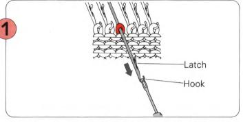
Place the eye of a single Transfer Tool over the needle hook, and pull the needle towards you until the stitch passes behind the latch.
