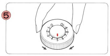
Set the Tension Dial according to the yarn you are using. (Refer to the Approximate Tension Chart on P.53).
