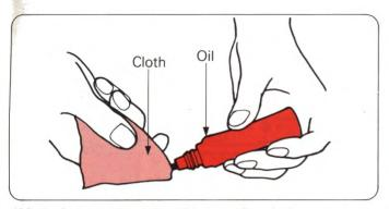
Wipe the metal parts with an oily cloth and clean plastic parts with a soft cloth and mild, neutral detergent.
