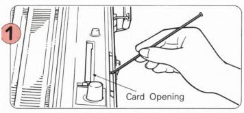
Insert the Punch Card Holder Pin in the hole behind the card opening.
