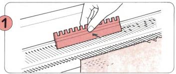
Replace any stitches that are on the stems of the needles back into the hooks and bring the needles (except those in E position) into B position.
