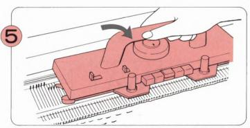
Lift up the K-Carriage towards you and remove it from the needlebed.
