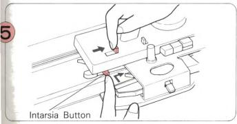
Set the Holding Cam Lever to I. To do this, slide the Holding Cam Lever to the right at the same time press in the Intarsia Button.
