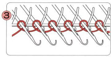
The loops should be behind the latches as shown.
