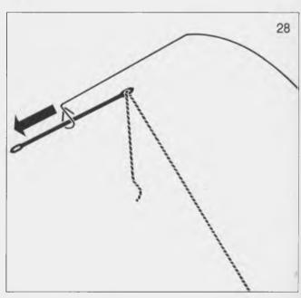
Now guide the bodkin from back to front through the eyelet at the tip of the tension arm.
