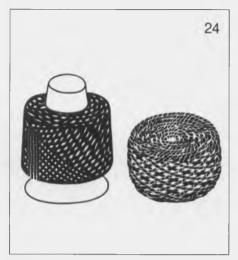
It is very important for the yarn to flow freely and smoothly. It will only do so if it has been wound into loose balls or on to cones.
