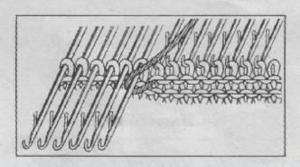
Pass the knitting yarn underneath the needle next to the last needle knitted as shown in left and knit one row.
