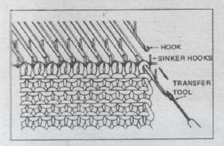
Push the needle back until the stitch is transferred be to the transfer tool.
