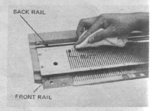
Apply oil to the knitting cams on the rear of the parriage (the obligue line), and wipe off excess oil with a rag.
