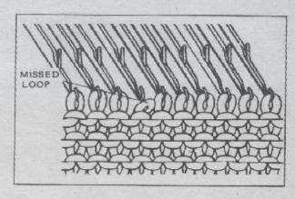
Insert a transfer tool into the loop just below the missed loop.
