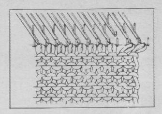
Pick up the stitch on the second row of the third stitches and transfer it to the empty needle. This increases one stitch.
