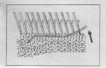
Pull the yarn up to the opposite side as shown by the arrow while pulling the knitted fabric lightly, and the stitches will be unraveled and the row beneath will be hooked on the needles. By repeating this process, unravel the incorrect rows. If the carriage is on the opposite side of the yarn end when the erroneous rows are unraveled, set the Tuck Lever and both knitting Levers at "EMPTY" position and slide the carriage to the side where yarn end is found.
