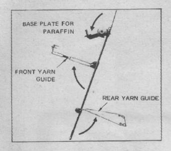
Pull out the front yarn guide, the rear yarn guide and the base plate for paraffin until they will stop, as indicated by arrow.
