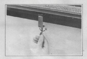
Insert the take-up rod with curved part down- wards into the hole at the back center of the machine.
