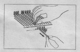
Push down the needle hook with the left hand, hold the butt and push it away from you.
