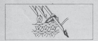
Wind yarn around hook of this needle > loosely, then by hand push the needle back to B position, thus making one stitch.
