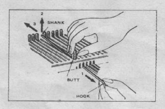
Pass the new needle through needle hole and pull it out toward you. Insert the shank in the needle bed. (Move the needle in the order 1, 2 and 3 as shown in left.)
