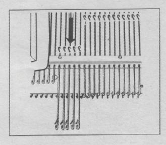
Wind the yarn round the respective needles pulled out to E position.
