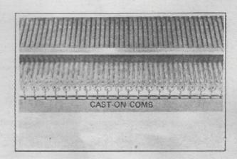
Set the knitting levers both sides to "PLAIN" > position, so that by sliding the carriage to the right or left the plain knitting can be done. Continuing to knit by sliding the carriage to the right or left, the carriage should be moved toward one side until a click can be heard and then moved toward the opposite side.
