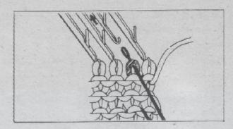
43. Hook this stitch onto the end needle and pull this needle through to E position.
