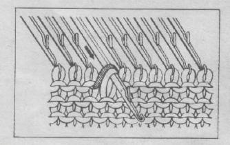
Move the needle at D position to C position. Then, hook the missed stitch on the needle hook and push the needle to B position to pick up the new loop.
