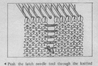
Unhook the latch needle tool, and pick up the loop with a transfer tool from the front and hook it on the needle.
