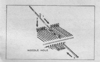
Pressing down the raised hooks of the needles, preturn the needle presser bar.
