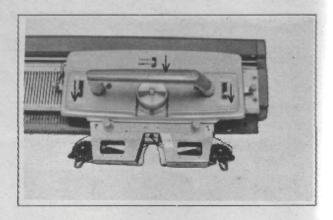
Pull down the yarn from beneath the rear yarn guide of the take-up rod to avoid end loops.
