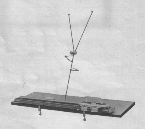
Install a clamp into clamping hole on the bottom be of the machine, secure it as indicated by the arrow. Then tighten the screw knob. Do the same with the other clamp.
