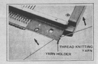
Place the thread knitting yarn on the latches of the needles in D position and hook the end of yarn on the yarn holder.
