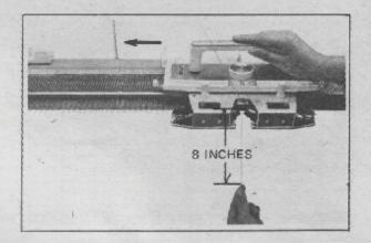
Yarn will pass over every second needle. Hook ▶ the cast-on comb onto the unknitted yarn in the front of the sinker hooks.
