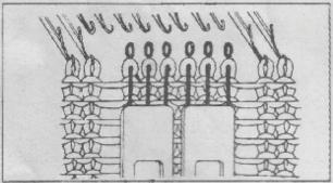
3. Loops on the left transfer tool are hooked on the empty latch needles at the right. (Fig. 3)
