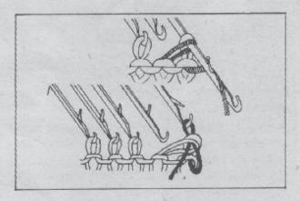
Transfer this stitch to the next inside needle, and push the empty needle to A position.
