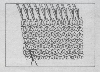
Unhook the knitted stitch on the latch needle with the needle tool inserted, and rip the stitches until just before the row on the latch needle tool by pulling down the fabric lightly with one hand and then by pulling down the latch needle tool with it inserted in the stitch firmly.
