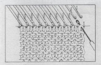
Hook the transfer tool to the next latch needle by moving the tool as indicated by arrow (1) and then pull it out slightly arrow (2).
