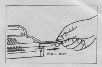
Pull the latch needle to be replaced out toward you to E position.
