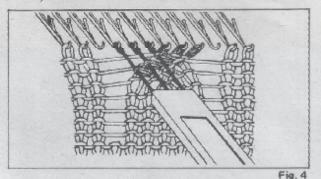
2. Transfer loops onto two transfer tools. (Fig. Transfer tools to be shown as parallel, not
