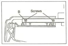
The place on which you put the Setting Plate on 9 mm Pitch Machine
