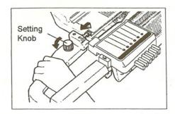
(2) Push the Release Button to return the Yarn Hook to resting position. Loosen the Setting Knob on the Setting Arm. While lifting up the Setting Arm on the side of the Setting Knob, pull out the Setting Arm.
