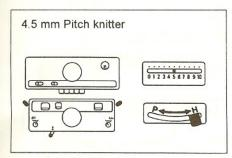
(1) Set the knitter and ribber as shown in the figure. Turn off the power switch. Set the Operation Lever on the Colour Changer to "" (non-working position).
