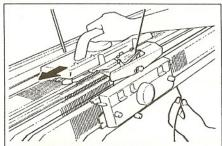
(8) While holding the yarn end, move the Carriages to the other side to cast on. Hang the Cast-on Comb and Weights.
