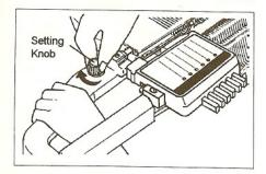
(3) Press the Setting Arm to the knitter, fasten the Setting Knob.
