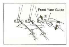
(4) Press down the Front Yarn Guide on the knitter and then remove the Yarn Tension Unit.
