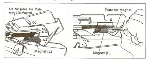
(2) Slide the Plate for Magnet onto the left Magnet from the edge until it fits with the margnet perfectly.
