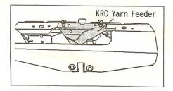
(2) Set the KRC Yarn Feeder to the Connecting Arm as shown in the figure. Then, fasten the screws.
