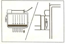
(10) Push the Changer Button No.1, the Yarn Hook will come up. Turn the Operation Lever to "▶" (working position).
