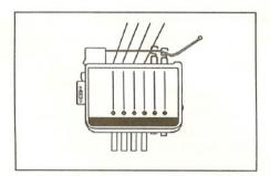
When the yarns do not come from the balls(corns) smoothly, two Yarn Hooks may come to working position and the Yarn Feeder may catch them together.
