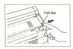
(3) After the Setting Arm is released, push the Felt Bar back which has been pushed out on the right side of the knitter.
