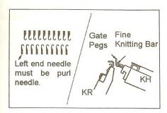
(2) Insert the Fine Knitting Bar behind the Gate Pegs on the knitter, so that it slips slightly underneath the needle bed. Aline both plain and purl needles in B position. (Bring forward a purl needle so that the left end needle is a purl needle and right end is a plain needle.) After operating the Carriages two or three times, place the Carriages on the right side.
