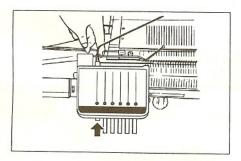
(5) Set Changer Button No.6 to working position by pushing it and hook the left end yarn onto the Yarn Hook. By pushing Changer Button No.5 the Yarn Hook No.6 will return to the resting position.
