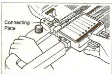
(2) Push the projecting part of the Connecting Plate against the end of the Felt Bar and insert it as far as possible.
