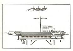
The figure shows the Colour Changer set up on the machine.
