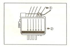
If the two Yarn Hooks come to working position... Return the yarn which is not knitted next into a corresponding Yarn Hook. Push the Release Button, and the Yarn Hook will return to the resting position.
