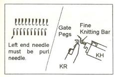
Insert the Fine Knitting Bar behind the Gate Pegs on the knitter, so that it slips slightly underneath the needle bed.
