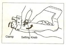
Loosen the Setting Knob as much as possible until the Connecting Clamp opens fully.
