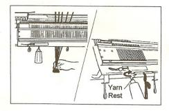
(4) Remove the ends of the left five yarns from the Yarn Clip, and tie five yarns together. Pass them between the Gate Pegs.
