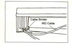
(11) Place the MD Cable behind the knitting machine. Fasten the MD Cable around the Setting Arm with Cable Binder so that the Carriage will not touch the Cable.
