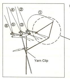
(3) Thread the yarn for yarn No.1 through the right Yarn Tension Unit, and hook the end of the yarn on the Yarn Clip.
