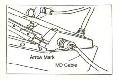
(12) Insert the other end of the MD Cable into the jack at the right end of the machine, matching both arrow marks.
