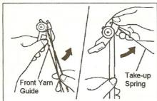
(5) Open the Front Yarn Guide in the direction of the arrow.
