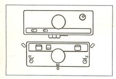
(4) Set the Carriages on the knitter and ribber as shown in the figure. Push  $\checkmark$  Key to load the knitting screen.
