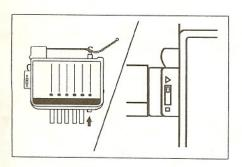
(5) Push Button No.1 so that the Yarn Hook will come up. Set the Operation Lever to "▶" (working position).
