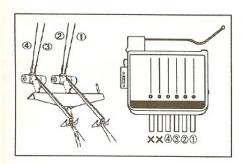
(1) When you thread four or fewer yarns, use two left Yarn Tension Units as shown in the figure. Thread the yarns into each corresponding hook on the Colour Changer. Thread four yarns into Yarn Hook No.1-4. Do not use Yarn Hook No.5 and 6. Follow the steps (1)-(8) on page 7-9 to knit full needle rib with yarn No.1.
