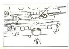
(7) Remove the right end yarn from the Yarn Clip and thread it into the Yarn Feeder.
